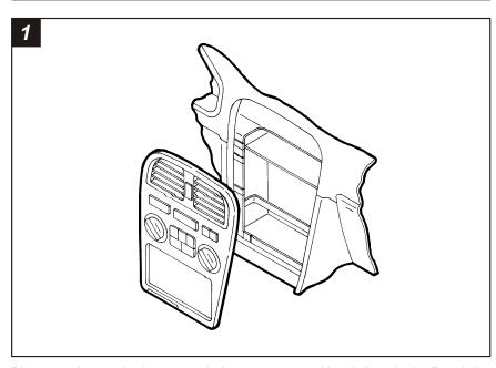
Disconnect the negative battery terminal to prevent an accidental short circuit. Detach the cable located under the left side of the glove box. Unclip the trim piece in front of the gear shifter and remove (2) Phillips screws exposed. Unclip the gear shifter trim and remove (2) Phillips screws exposed. Unclip the radio trim bezel and remove. Remove (6) Phillips screws securing the factory head unit and disconnect the wiring.
